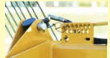
Single pin gearbox cam adjustment to adjust windrow formation for a variety of crop conditions
