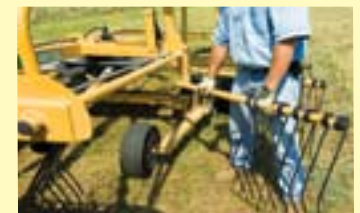
Removable tine carriers (with storage location) for narrow transport
