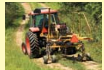
Flip up protection frame for narrow transport
